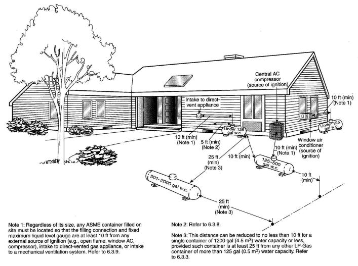
FIGURE I.1(b) Aboveground ASME Containers. (Figure for illustrative purposes only; code shall govern.)
